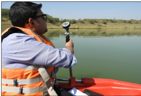
Data collection for river velocity from Parvati river, Sheopur, using Water flow Probe
