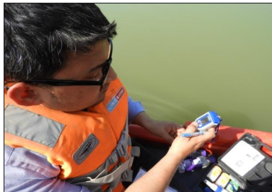
Water quality analysis using portable instruments
